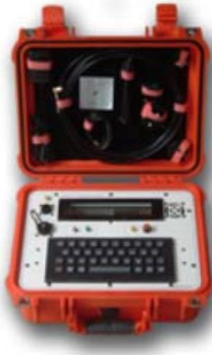
*Chatty Beetle Terminal. A terminal is the orange box unit. It sends and receives short text messages via Iridium Short Burst Data (SDB) service. Control terminals are identical to field / normal terminals, except that control terminals are given special permissions to send alerts and other functions.*
